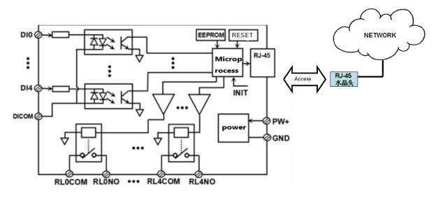
Figure 2 WJ95-RJ45 Block Diagram
