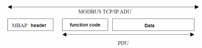
Figure 6: MODBUS request/response over TCP/IP
